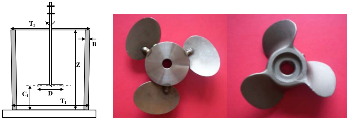
Fig. 1: Mixing vessel (T1) and impellers studied (Maxflo on the left and the marine impeller on the right)
